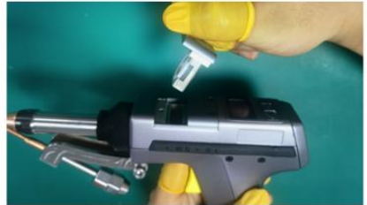
② Remove the protective lens holder
